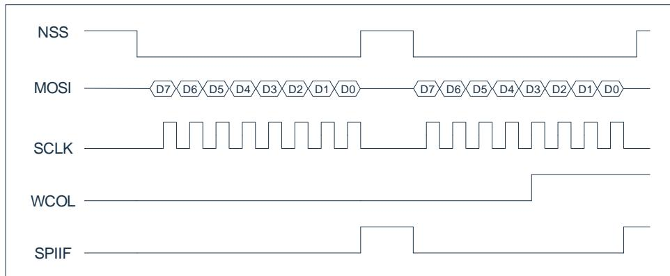
The specific conditions for the write conflict are: during data transmission, when NSS is low, the first From the time when a data is sent to the eighth falling edge of SCLK, if SPDR is written during this period, a write conflict will occur and WCOL will be set to 1.
