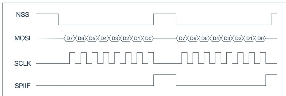
When SSCEN=0, configure the SPI clock polarity CPOL=0, clock phase CPHA=0, the slave selection line is used as shown in the figure below:
