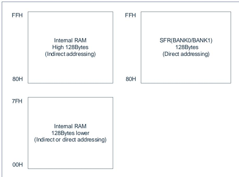
The high 128 bytes and SFR shown in the figure above occupy the same area (80H~FFH), but they are independent. Directly address the storage space (SFR) higher than 7FH and indirectly address the storage space higher than 7FH (high 128 bytes) into different storage spaces. SFR is divided into two pages, BANK0 and BANK1, each page is 128Bytes, occupying the same address area, and entering different storage spaces through the paging register selection.
