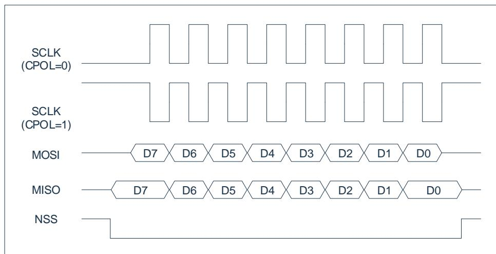
When CPHA=0, the NSS line must be de-set and reset between each successive serial byte. In addition, if the slave writes data to the SPI data register (SPDR) when NSS is at low level, a write conflict error will occur. When CPHA = 1, the NSS line may remain low between consecutive transmissions (it can always remain low). In a system with a single fixed master and a single slave driving the MISO data line, this format is sometimes preferred.
