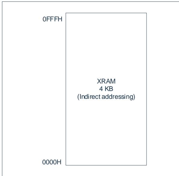
XRAM/XSFR space access is operated by the DPTR data pointer. DPTR includes two sets of pointers: DPTR0, DPTR1, which are selected by the DPS register. For example, through MOVX indirect addressing operation, the assembly code is as follows:
