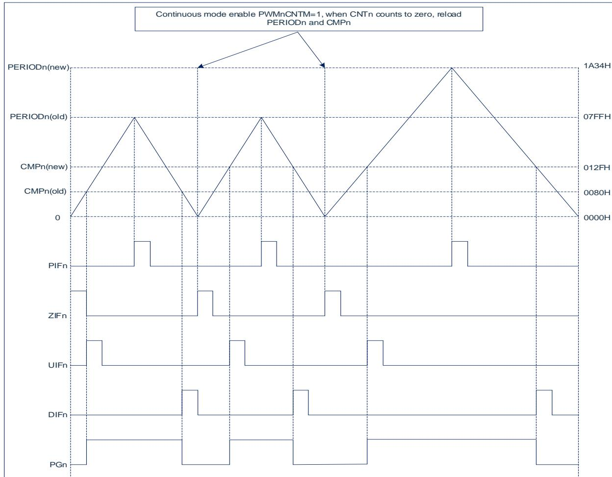
The center-aligned counter waveform (symmetric counting) is shown in the figure below:
