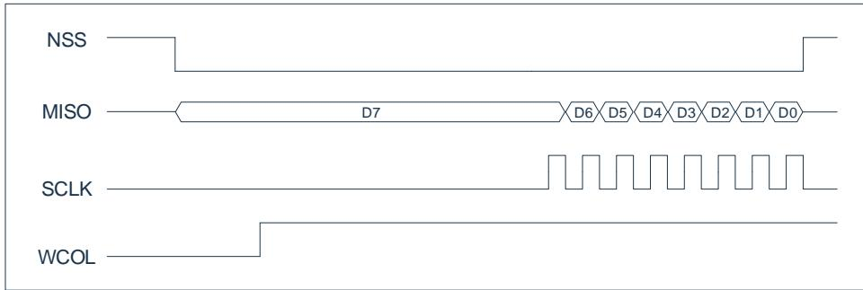
In addition, after writing SPDR in the slave mode, the NSS controlled by the host does not immediately become low. When NSS is low, you need to wait for the second edge of SCLK to start before entering the real data transmission state.
