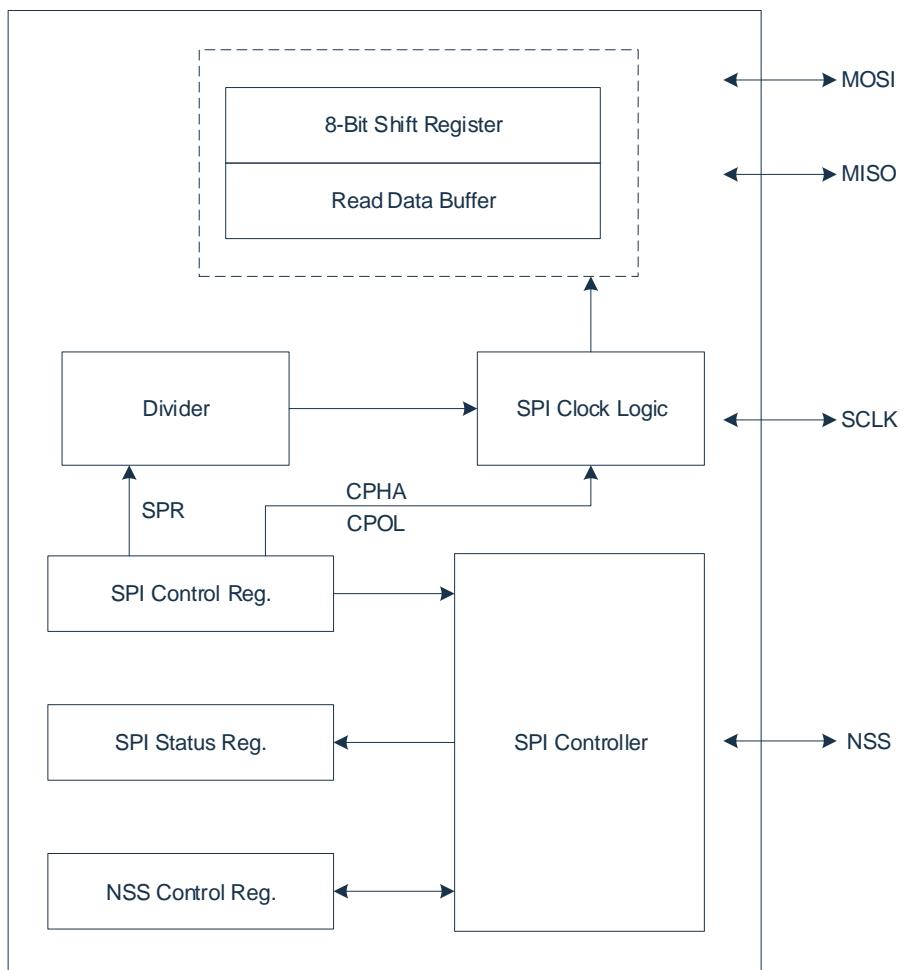
The pins associated with SPI are: NSS, SCLK, MOSI, MISO.
