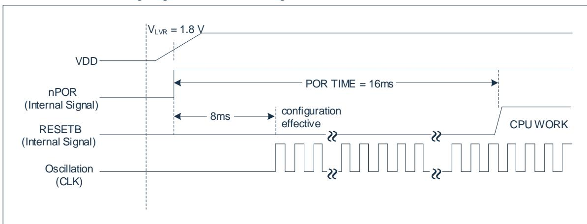
Whether the system is power-on reset can be judged by PORF (WDCON.6) flag bit. The reset types that can set the PORF flag to 1 are: Power-on reset, LVR reset, External reset, CONFIG protection reset.
