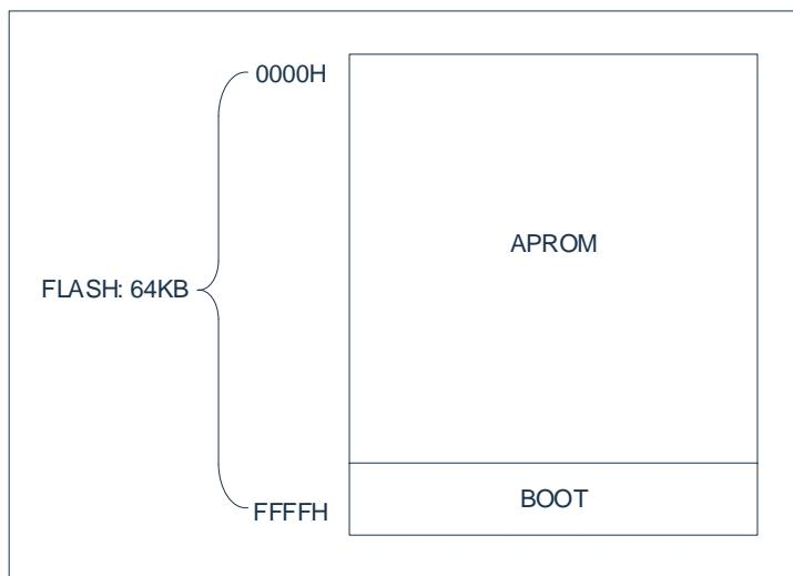
After the chip is reset, the CPU starts to execute from 0000H. Each interrupt is assigned a fixed address in the program memory, and the interrupt causes the CPU to jump to this address and start executing the service program.
