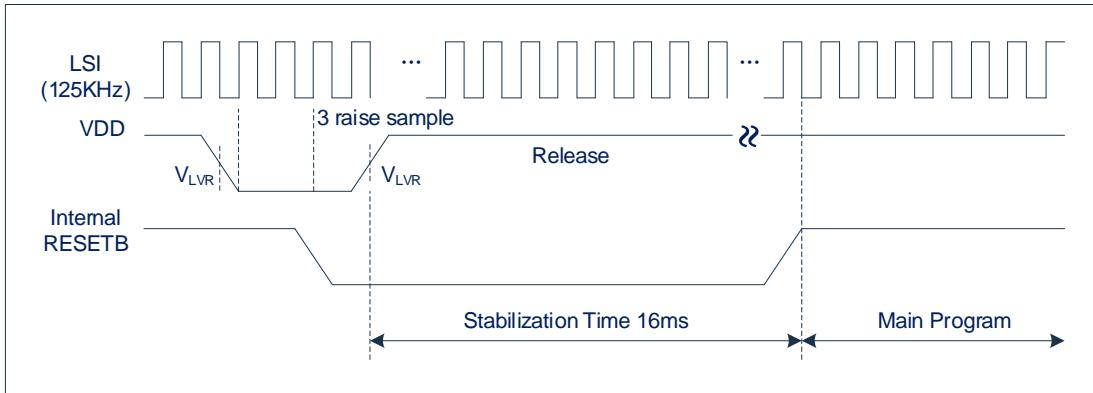
The chip reconfiguration process within the Stabilization Time is the same as the Power-on reset configuration process.
